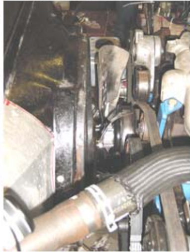
Of course I forgot that the multi belt drives the fan the other way, so the fan ate the belt
