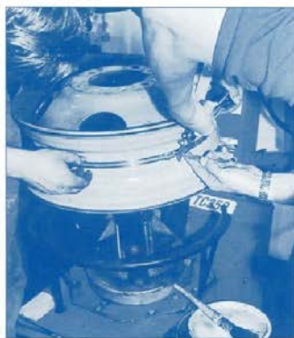
The counterweight plate and the sensor are mounted using a large stainless-steel clamp. Excess strap is cut off.
