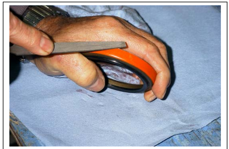
Fig. 26. Using a file to chamfer metal edge of inner seal.
