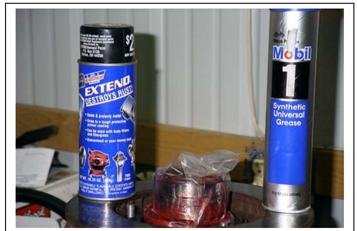
Fig. 1. Permatex Extend on the left and Mobil 1 tube of synthetic grease on the right used to pack bearings.
