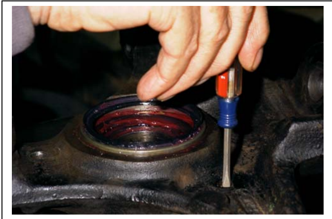
Fig. 23. Threading inner grease seal retainer plate bolt in place.
