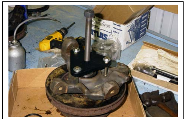
Fig. 9. Warner bearing puller tool knuckle puller plate bolted in place shown with puller screw in place.
