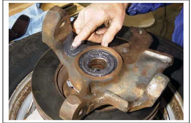
Fig. 25. Packing bolt holes with grease.
