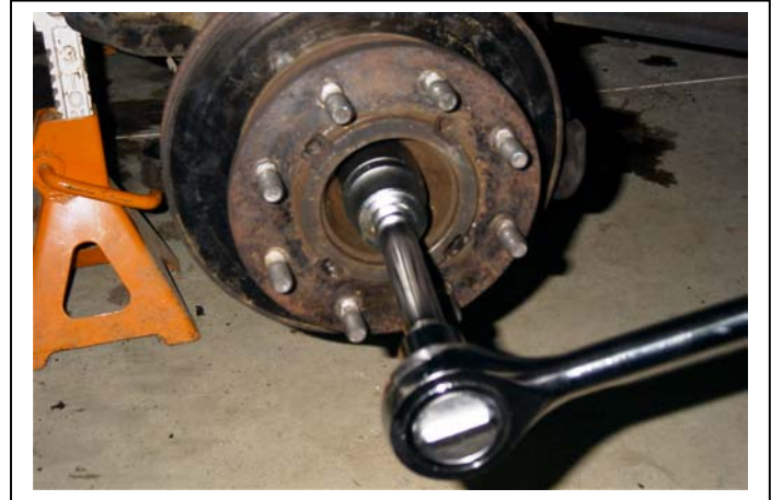
Fig. 28. Axle nut being tightened.
