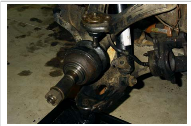
Fig. 13. This picture illustrates both the upper and lower control arms as well as the
