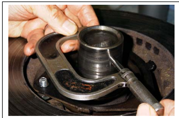
Fig. 11. Caliper being used to measure hub shaft dimension.
