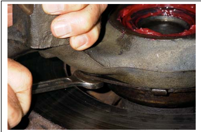
Fig. 24. Inner grease seal retainer bolt being tightened.
