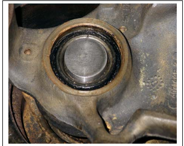
Fig. 8. Circular Warner puller tool plate (aka “puck”) placed over end of hub shaft. Puller screw point bears on this plate when pulling the knuckle off the hub.
