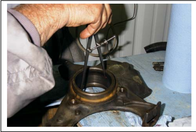
Fig. 12. Measuring bore of knuckle with caliper.
