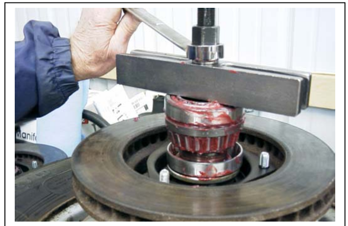
Fig. 22. Pressing bearings onto hub shaft by turning nut on the forcing screw with a wrench.
