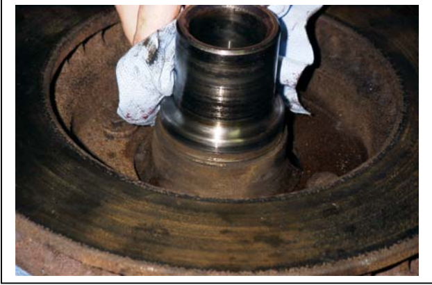
Fig. 15. Cleaning hub shaft.
