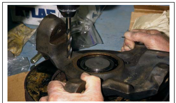
Fig 5 This photo illustrates enlargement of inner grease seal retainer plate threaded bolt holes in the knuckle when needed.
