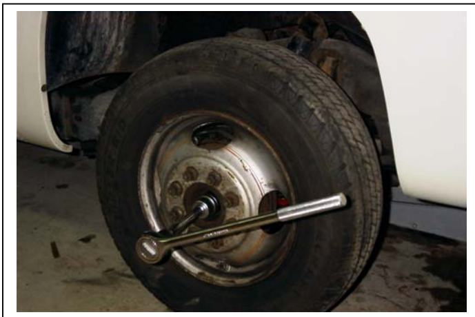
Fig. 2. Note \frac{3}{4} " drive ratchet with extension and 1-1/2" socket over drive axle nut. Turn wrench in conventional counterclockwise direction to loosen nut, both driver and passenger sides.
