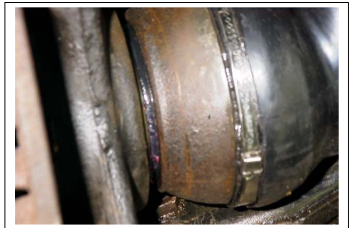
Fig. 29. Tightening axle nut draws the outer CV joint, seen on the right side above, in close proximity to back side of the knuckle, on the left side, and in the process seats the inner grease seal lips.
