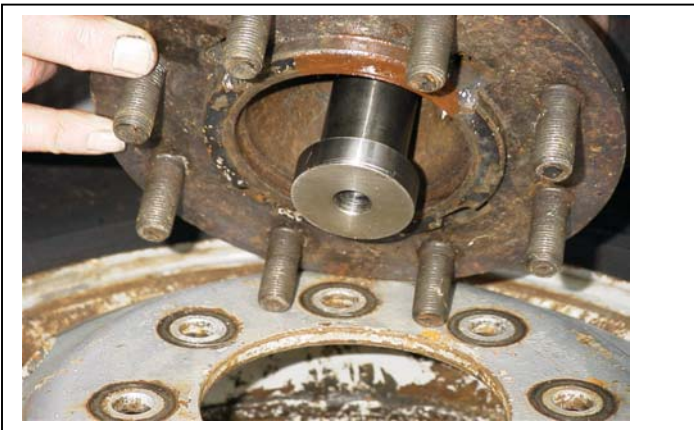
Fig. 20. Axle cavity pressing screw retainer.
