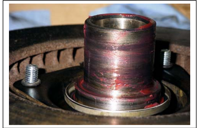
Fig. 17. Seal (outer) retainer plate, with bolts in place, and outer seal in place over hub shaft. Note hub shaft bearing stop shoulder just above seal as well as light coating of grease on hub shaft.
