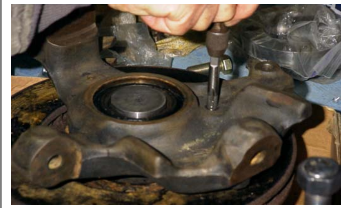
Fig. 6. Chasing grease seal retainer plate bolt hole threads in the knuckle.
