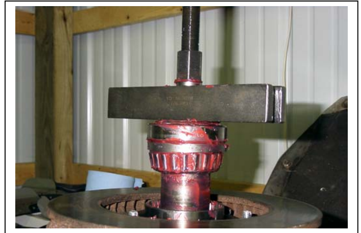
Fig. 21. Bearings stacked on top of hub shaft. Note OTC puller bar and pressing/forcing screw in place on the shaft.
