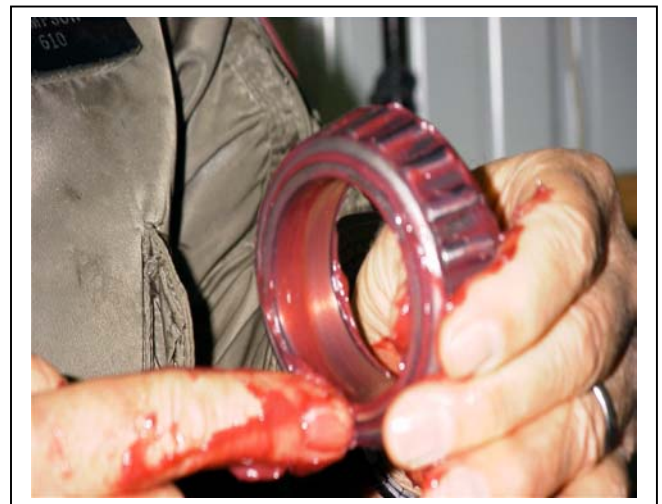
Fig. 18. Bearing being packed with grease.
