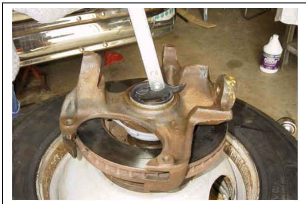
Fig. 7. Inner grease seal removal.
