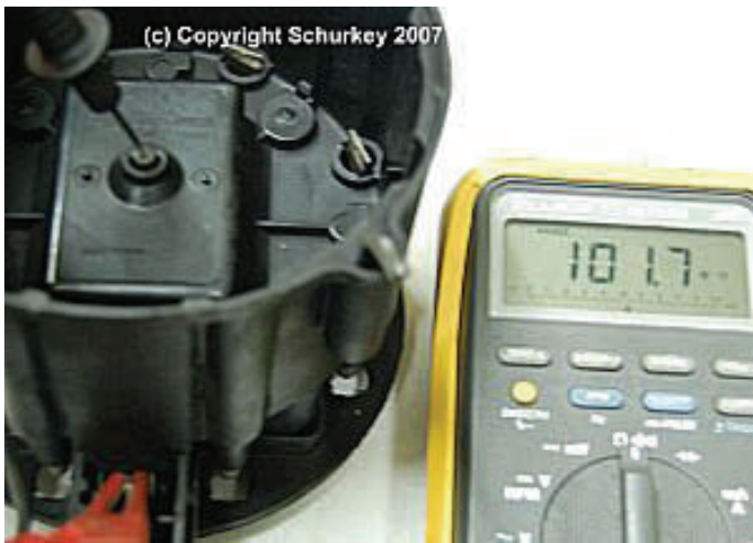
Photo 18. Middle blade to carbon button. Meter shows 101.7 Megohms—very high resistance. Some coils will have NO continuity—open circuit. That can be OK.
