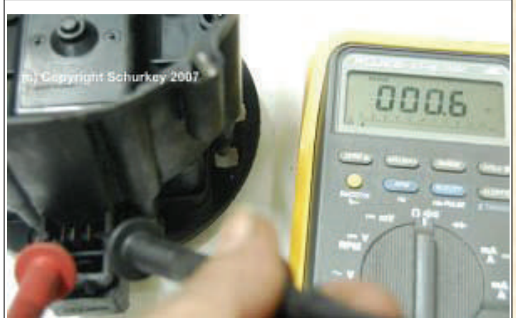
Photo 16. Testing B+ to C- (coil primary) continuity. Meter shows 0.6 ohms.
