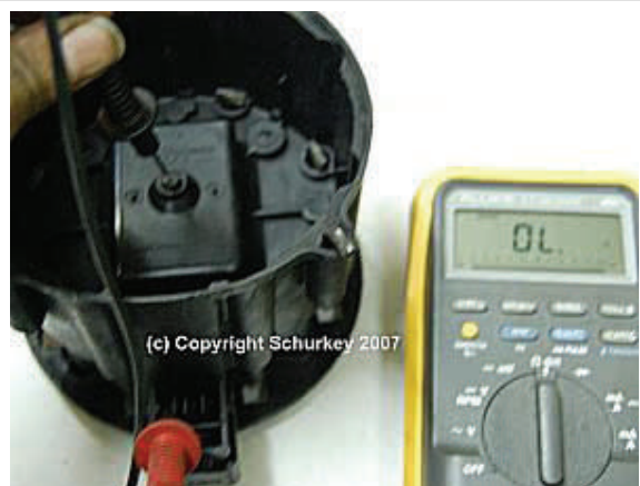
Photo 17. B+ to Carbon Button. Meter shows "Open Loop" (open circuit—no continuity) (Some coils may have continuity—that's ok too.)
