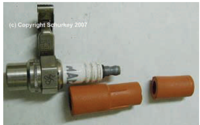
Photo 10. HEI Spark tester and cut-off spark plug boot used as a support tool.
