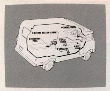
Models B and BL represent the second generation of Thermasan Waste Destruction Systems and replace the original Thermasan Model A (for motorhomes).
