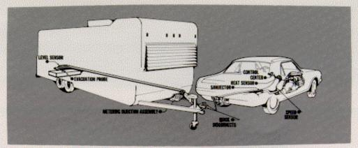
Models BT and BLT are also members of the second generation of Thermasan Waste Destruction Systems. Since Truck Campers and Travel Trailers must be towed by or mounted on another vehicle for mobility, Models BT and BLT come with specially designed, sanitary and electrical, quick disconnect fittings to link the waste transfer mechanism to the control and incineration components. Except for this one addition, the Models BT and BLT perform exactly like Models B and BL.
