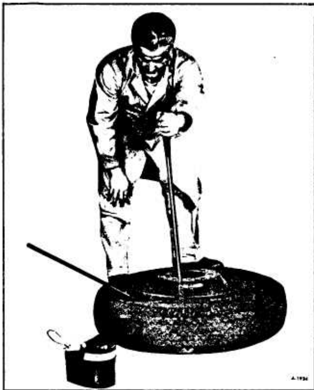
Figure 8—Inserting Tire Iron to Lift Bead
