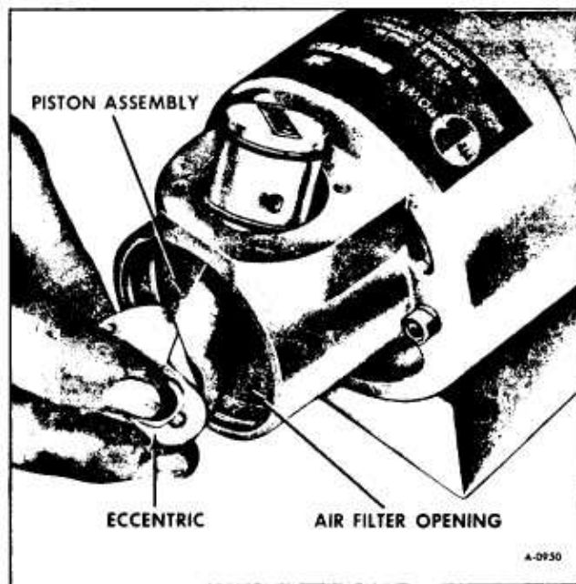
Figure 28—Removing Compressor Piston
