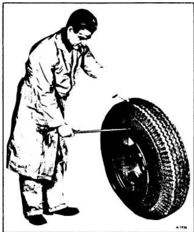
Figure 10—Inserting Tire Iron in Second Bead
