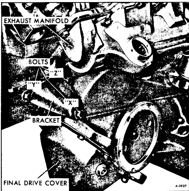
Figure 15—Disconnecting Final Drive From Engine
