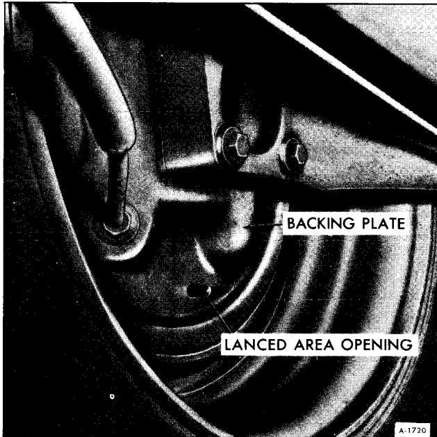
Figure 6-Lanced Area in Backing Plate
