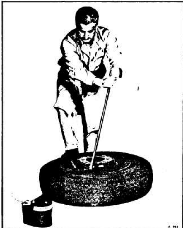
Figure 9—Lifting Bead Over Rim
