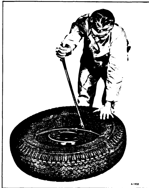
Figure 6—Working Bead Onto Rim
