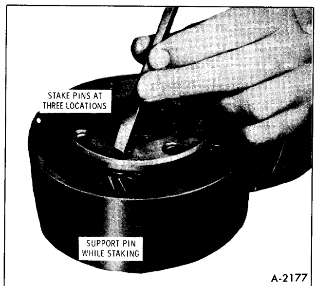
Figure 60—Staking Pinion Pin
