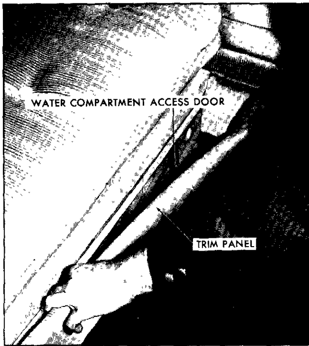
Access to Water Pump and Controls
