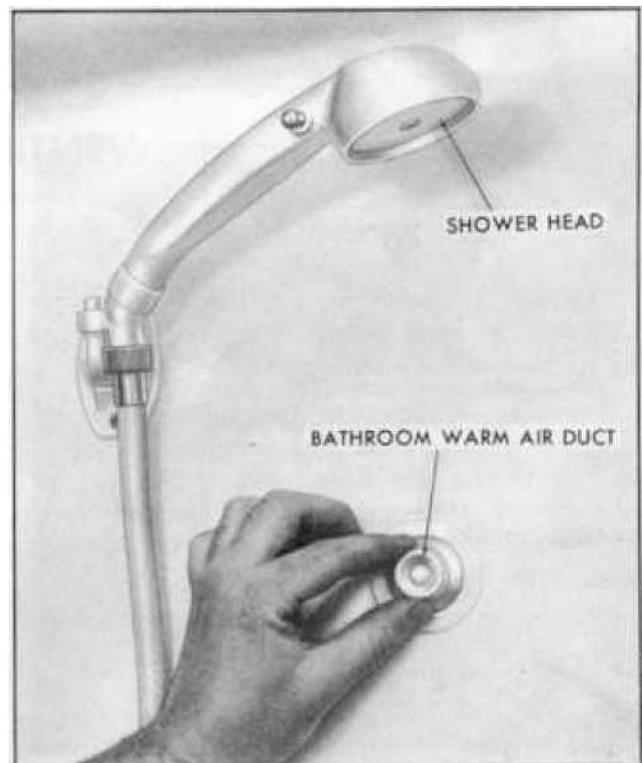
Bathroom Warm Air Duct (Type 1)
