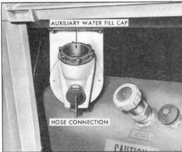
Location for Filling Water Tank (Type 1)
