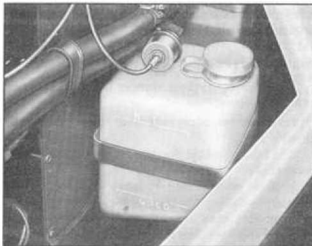
Coolant Recovery Tank
