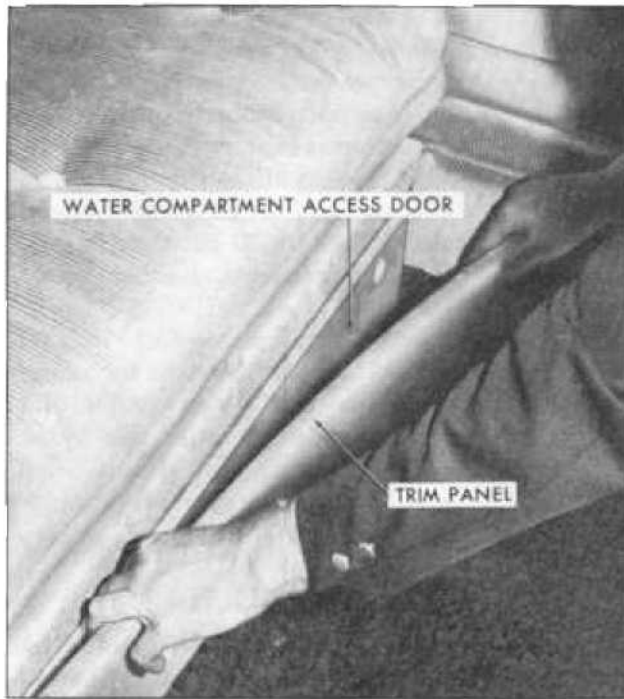
Access to Water Pump and Controls
