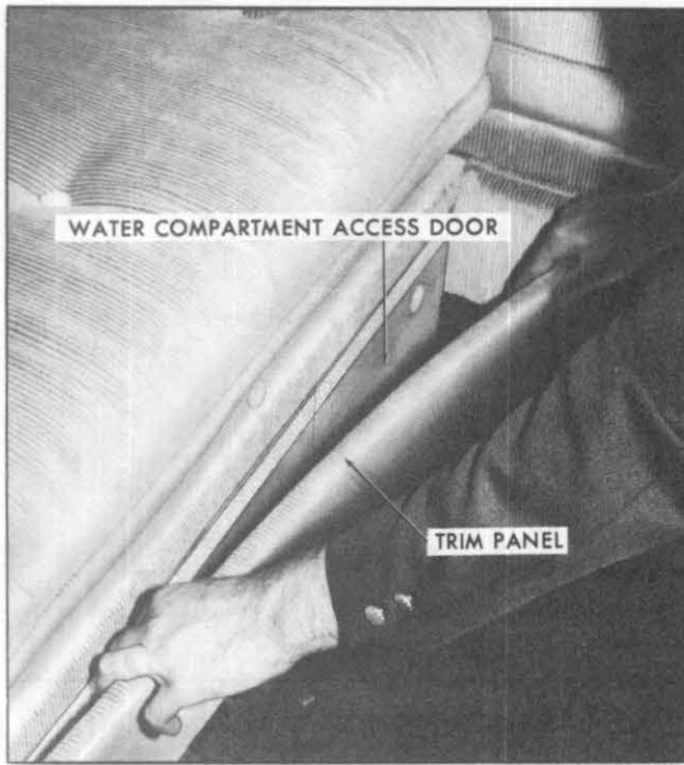
Access to Water Pump and Controls (ZEO 6581)
