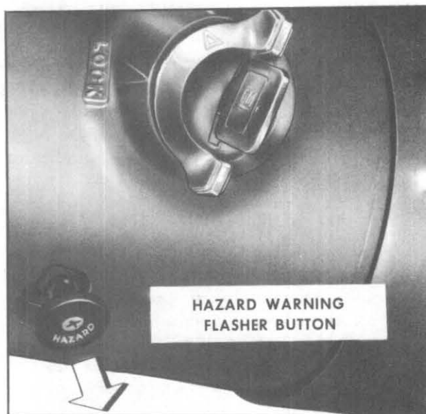
Hazard Warning Flasher
