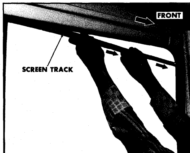
Removing Screen Track (Typical)
